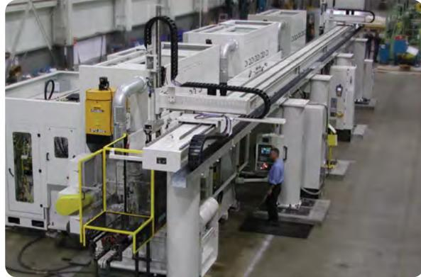
A custom enclosure system protecting the operator from the machine tool and the moving parts of their production line.
