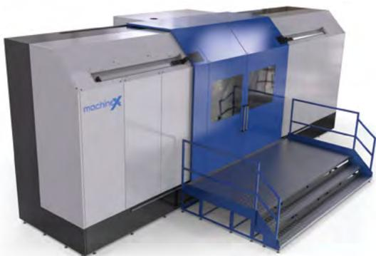
Enclosure for a large cylindrical roll grinder.
