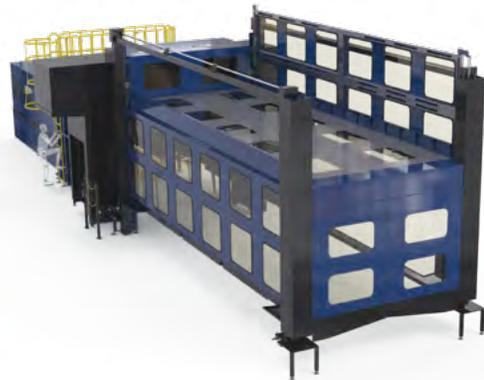
A custom pallet door system allows for loading and unloading of large parts.
